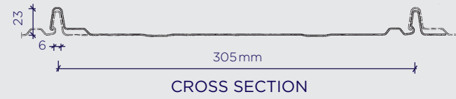
Smart Tray™ Snap Lock 0.7mm Aluminium Roof.
